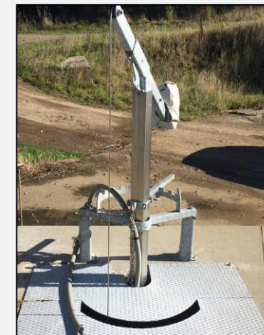
*Landia's manure mixer is an all-round, efficient, and solid mixer. The low rotation speed makes it very suitable for mixing even very thick manure.*
