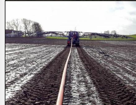
*SDS 8000 is a ground-breaking model with new functions such as hose crane arm, electro-hydraulic hose winding control, electrical tire pressure adjustment, and return pumping of slurry*
