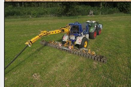
*SRS 1200: Slurry is being pumped directly to the machine sparing transportation costs. Low weight means entering fields at an earlier stage*
